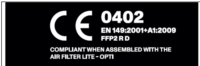
Picture of marking on mask skin Air Mask Lite
